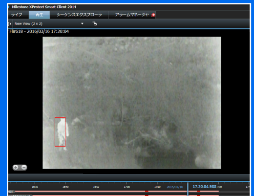
savVi detecting a person loitering at one of the dam sites, displayed in Milestone Smart Client
